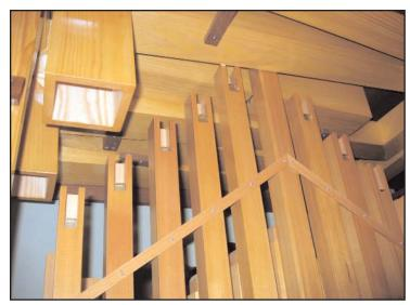
Figure 2. This view of the interior shows the accompaniment cello pipes in the foreground and overhead, the trombone resonators.
